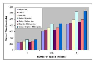
Figure 12: Overhead and scalability of Select queries for different extensions
