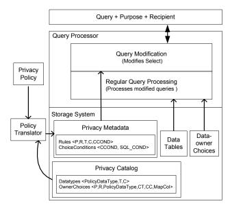
Figure 1: Unified original architecture for limiting disclosure
