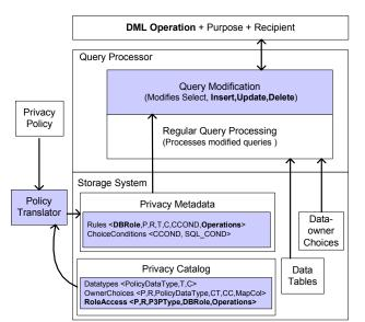
Figure 5: Architecture after first two extensions
