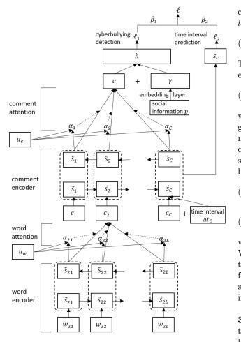
Figure 2: Hierarchical Attention Networks for Cyberbullying Detection.
